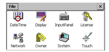
The settings for date/time, display and touch are already factory set for optimum performance. The network settings, however, must always be adapted to the network in place.
